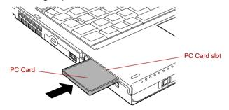
Figure 3-1 Inserting the PC Card
